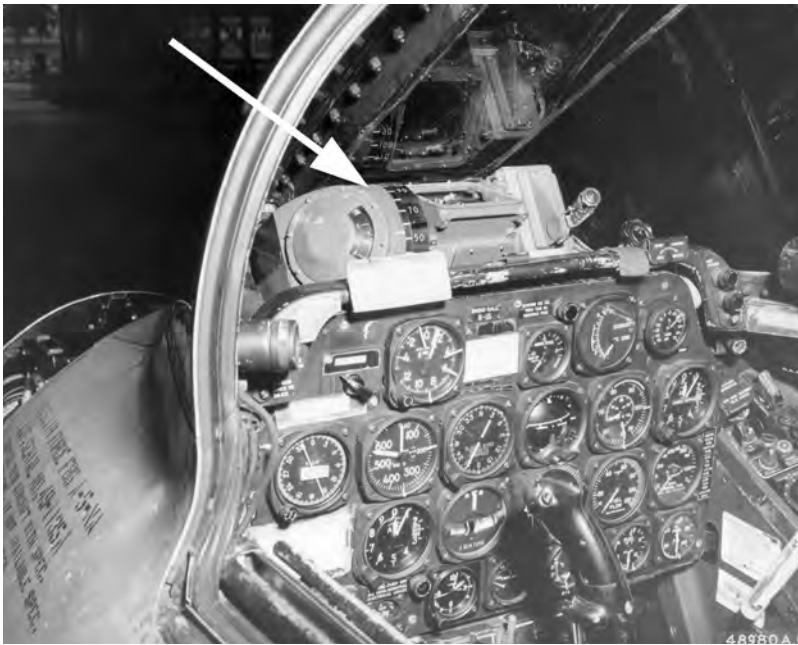
Cockpit photograph of North American F-86A Sabre taken on July 26, 1950, showing cockpit instruments and A-1C(M) gunsight. The A-1C(M) was added to the second production run of F-86s. (National Archives)
